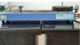
Twist is the estimation of the spiral turns given to a yarn in order to hold the element of the fibers on thread together.
