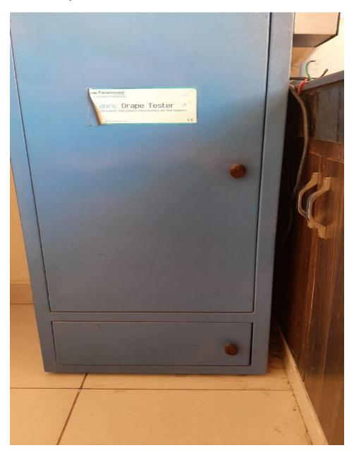
Cusick drape test is measured the drape property of fabric on the basis of its sheer and bending stiffness properties under motion.
