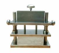
Perspiration is usually liable for the change in color of the material. It's testing equipment which is employed to work out color fastness of dyed or printed fabric against perspiration thanks to water, sea water etc. and sublimations during storage. It's carried on by exposing the material sample to the action of the both acidic and alkaline medium during a controlled temperature and pressure alongside an undyed sample.
