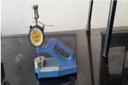
The fabric thickness is usually measured as the distance between the two fabric surfaces under a certain level of applied pressure, depending on whether nonwovens are high loft.
