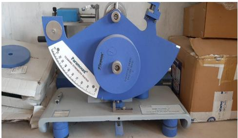
Textile Elmendorf Tearing Tester also a kind of textile testing equipment, to determine the ballistic tearing strength of woven fabrics, plastic films, paper, Textile Elmendorf Tearing or other similar materials.
