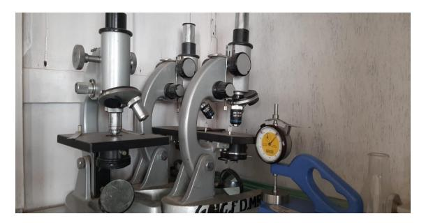
Microscope is used to closely analyse substances to understand their composition. We have seen this equipment used widely in the medical field, but every microscope is different and poses different qualities for various researches. However, in the textile industry it is mainly used to understand the weave pattern with which the fabric is woven. It is also used to understand the
