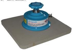
GSM means gram by square meter, and the weight of the textile which includes both knit, woven and non-woven is the designation, as the name implies. It's a basic tool used to cut a tissue sample for the measurement of the GSM of the textile. The measurement of the fabric is 11.2 cm in diameter. The sample shall be measured and computed for GSM after cutting.
